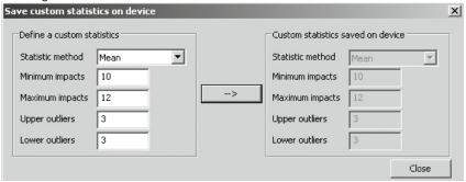
Define the statistics method as desired and load this setting onto the RockSchmidt by clicking on the arrow in the center of the window.
