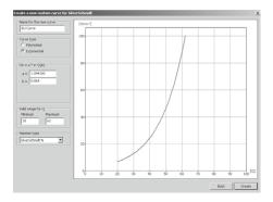
Type in the name for the new curve and enter the parameters and the hammer type (RockSchmidt N) for which it is applicable.
