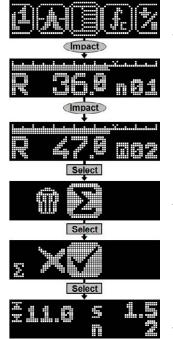
'R' is automatically set as the unit for this method as no correlation is made to UCS or E-modulus.
