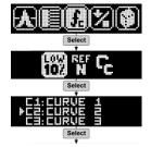
Reduced dispersion and direct conversion to compressive strength based on validated curves, regional curves or user defined curves bring improved accuracy to compressive strength estimates.
